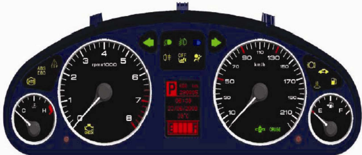
Telltale indicated by LED (Green: 6ea / Blue 1ea / Yellow: 11ea / Red: 1ea / Spare box: 2ea)
