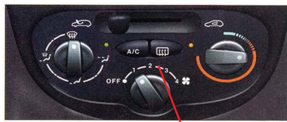
AC / Heater Control Panel
